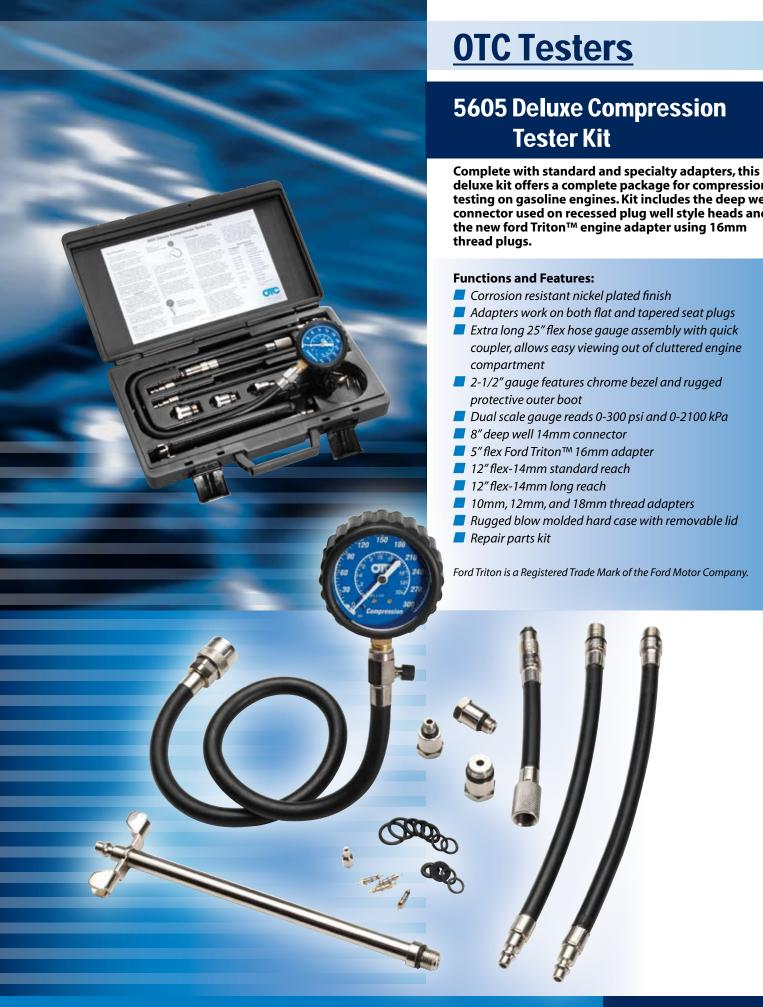
deluxe kit offers a complete package for compression testing on gasoline engines. Kit includes the deep well connector used on recessed plug well style heads and the new ford Triton™ engine adapter using 16mm
