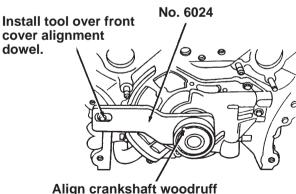
Align crankshaft woodruft key with keyway on tool.
