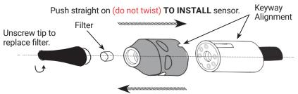
Pull straight out (do not twist) TO REMOVE sensor.
