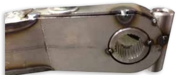
Pro Fabricator Link Arm tacked together
