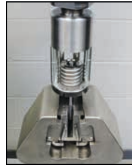
Retainer pull-through testing
