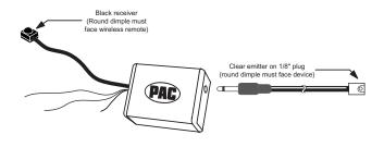
\* note: The IR remote being used must use a 40kHz or 56kHz carrier frequency. Consult with equipment manufacture to determine the carrier frequency. Check website for known units that do not work.
