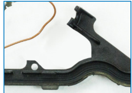
19D: Finished Modified Gasket
