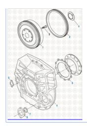
**Cummins Engine 2017** Flywheel Assembly - L10 / M11 / ISM Series
