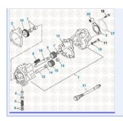
**Cummins Engine 2017** Oil Pump Assembly - N14 Series
