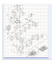
**Cummins Engine 2017** Turbocharger and Exhaust Manifold - 6C / ISC / ISL Series
