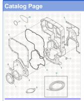
**Cummins Engine 2017** Front Cover Components - ISX Series
