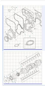
**Cummins Engine 2017** Front Cover Components - ISX Series
