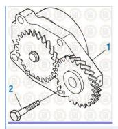
**Cummins Engine 2017** Oil Pump - 6B Series
