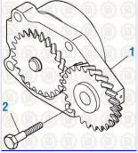
**Cummins Engine 2017** Oil Pump - ISB / QSB Series
