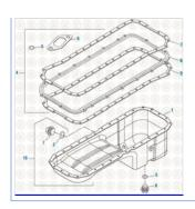
**Cummins Engine 2017** Oil Pan - ISB / QSB Series
