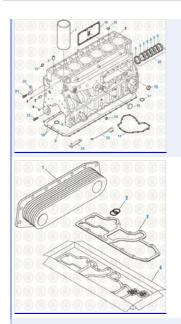
Caterpillar Engine 2019 Cylinder Block - 3100 / C7 Series
