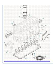
**International Engine 2019** Cylinder Block Components - DT-466E / DT-530E (1993-1999 HEUI)
