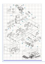
**Detroit Diesel Engine 2019** Exhaust Manifold and EGR Cooler - Series 60
