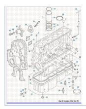
**Detroit Diesel Engine 2019** Cylinder Block and Oil Pan Components - Series 60
