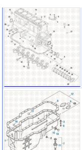
**Volvo / Renault Engine Components 2015**Cylinder Block Components - Renault / E-Tech
