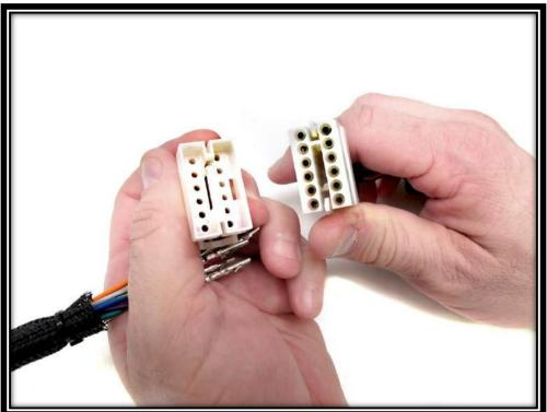
Step 15: Insert the newly pinned wires into the 12-pin connector housing. Make sure, while inserting the pins, that once connected the wire matches the one across from it. The diagram on page 11 illustrates the pinout of the 12-pin connector housing from the wire side.
