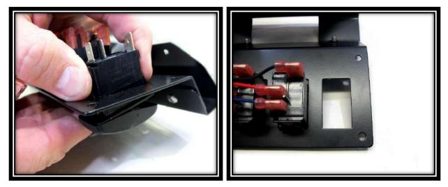
**Step 24:** Insert the **Winch Control Add-on Switch** into the empty socket of the bracket.
