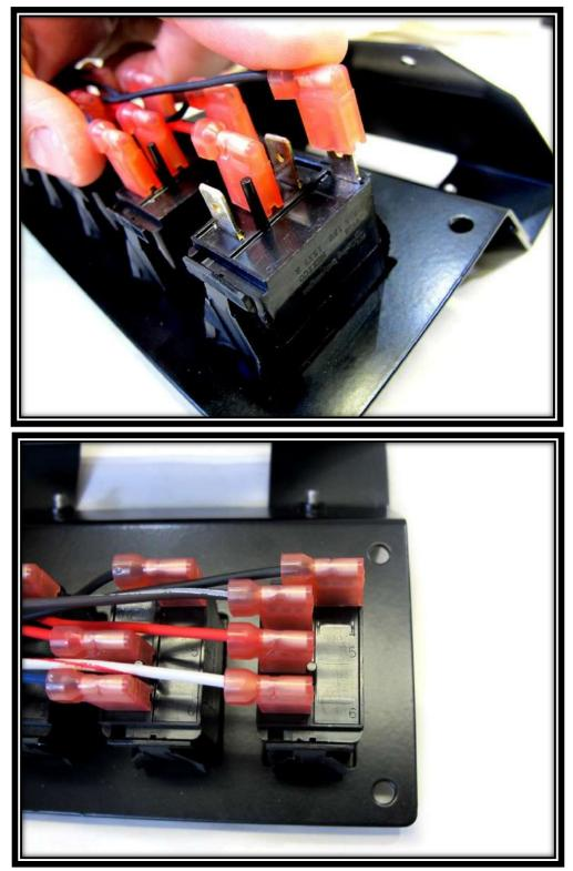
Step 27: Strip and terminate the other ends of the wire as you did in Steps 13 – 15. And insert the WHITE/RED into slot #9 of the 12pin connector shell and the BROWN/WHITE into slot #10.
