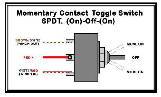
Step 26: Reconnect the power, ground, and Switch Panel wires to the Winch Control Add-on Switch as seen below.
