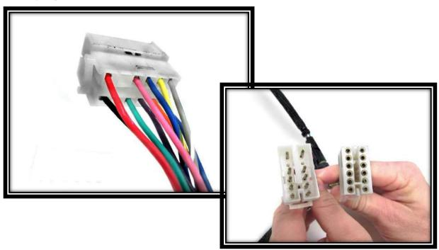
**Step 17:** Link the two connectors and join the wiring harness from the **Fuse/Relay Center** to the **Switch Panel**. Use **zip-ties** to secure the wires up under the dash and out of the way.
