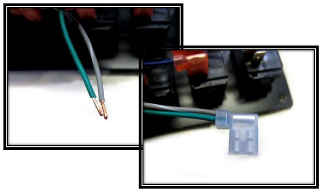
**Step 21:** With both wires inside, crimp the terminal, and reconnect the doubled **Switch Panel wires** to the switch.
