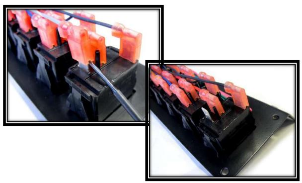
**Step 19:** With the **Switch Panel wire** removed from the switch, cut off the terminal, and strip the wire <sup>1</sup>/<sub>4</sub><sup>"</sup>.
