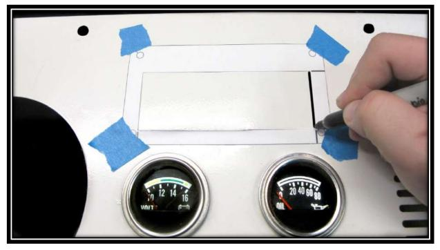
**Step 4:** Then, use your cutting tool to make the appropriate sized hole.
