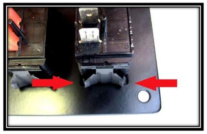
**Step 23:** These tabs lock the switch in place. To remove the switch, squeeze the tabs in and slide it out of the bracket.
