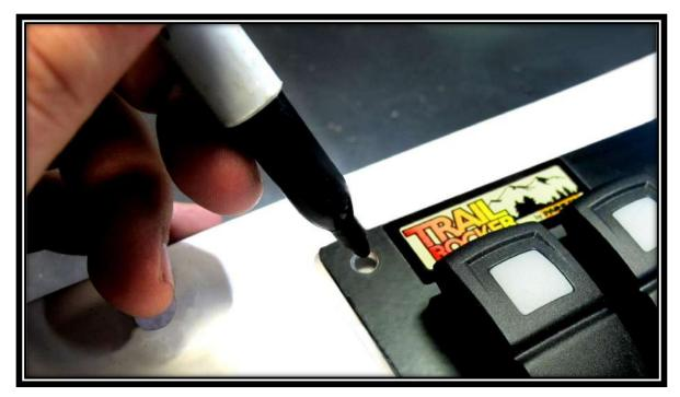
**Step 8:** Remove the **Switch Panel** and use a  $\frac{5}{32}$ " drill bit to create the (4) mounting holes.
