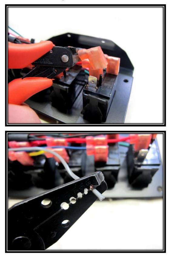
**Step 20:** Take the **Switch Panel wire** you just stripped and one of the additional **Switch Panel wires** included in the kit; then slide them together into a 16-14 ga. terminal provided in the included parts kit.
