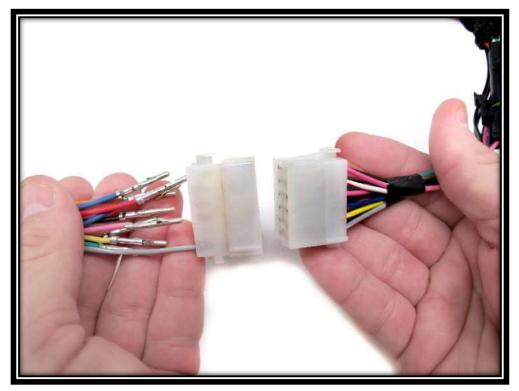
Step 16: Once completed, the connector should appear as it does below. The 2 empty cavities are for optional winch wires (see page 17).
