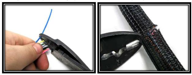
Step 13: Strip each of the Switch Panel Wires <sup>3</sup>/<sub>16</sub>", and install a male pin terminal from the parts kit onto the end of each wire. See page 4 for detailed instructions of how to properly crimp these terminals. We recommend Painless #70900 Roll-Over Crimpers.
