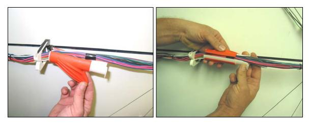
The wire is inserted into the tool. The tool is then closed around the wire
