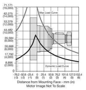
The maximum load curve is defined by bearing static load capacity. This curve should not be exceeded at any time including shock loads.
