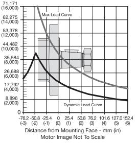
The dynamic side load curve is based on unidirectional steady state loads for L<sub>10</sub> bearing life at 3 x 10<sup>6</sup> revolutions.
