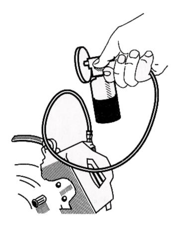
WARNING! Brake fluid is corrosive. Avoid contact with painted surfaces, clothing, skin and eyes. Wear eye protection. Follow vehicle manufacturer's sequence order for bleeding brake lines If you jack vehicle up, BE SURE TO USE JACK STANDS!
