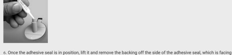
the glass of the windshield, opposite the upwardly pointing tab. Then, press the adhesive seal onto the glass surrounding the PIT. The PIT must continue to be positioned within the adhesive seal's central hole and the adhesive seal's tab must be pointing upward.
