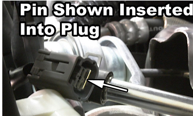
Pin shown inserted into PCV diagnosis harness.
