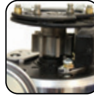
Precision magnetic pickup coil and reluctor.
