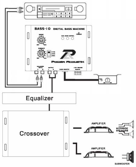
**NOTE:** For signal connection, the output RCA connectors should be connected to the next component after the BASS-10, such as a crossover, equalizer, or amplifier. Just remember, the BASS-10 should go inline before a crossover.
