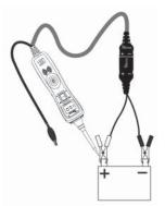
While the PP3 is in Power Probe Mode, contact the probe tip to a <u>POSITIVE</u> circuit. The red positive sign "+" LED will light and the voltage reading of the circuit will be indicated on the LCD display. If the audio feature is turned on, a high pitched tone will sound.
