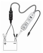
While the PP3 is in Power Probe Mode. Contact the probe tip to a <u>NEGATIVE</u> circuit. The green negative sign "" LED will light. If the audio feature is turned on, a low pitched tone will sound.
