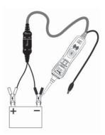
While the PP3 is in Power Probe Mode. Contact the probe tip to a <a href="MEGATIVE">MEGATIVE</a> circuit. The green negative sign "- " LED will light. If the audio feature is turned on, a low pitched tone will sound.
