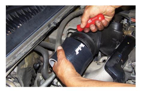
**STEP 14**Fit the silicone hose to the intake duct.
