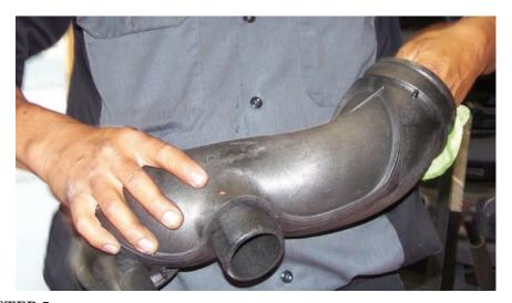
**STEP 5**Wipe out the interior of the inlet duct.
