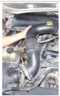
**STEP 2**Un-clamp OEM intake duct hose and set to the side.
