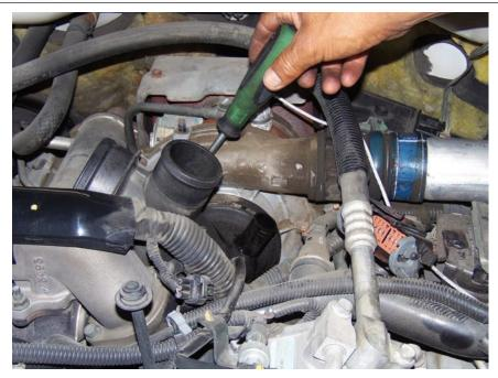
**STEP 3**Remove V-Band clamp and inlet duct.
