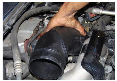
**STEP 7**Place intake duct into position.
