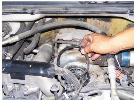
**STEP 4**Remove inlet duct seal, be careful for it may be hot.
