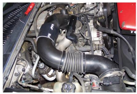
**STEP 15**Fit the other hose into the open end of the cut silicone hose.
