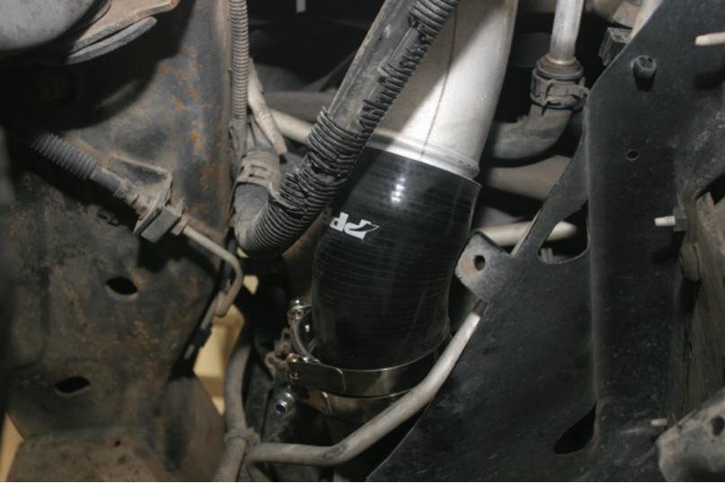
Step 13: The clamps are installed and tightened.
