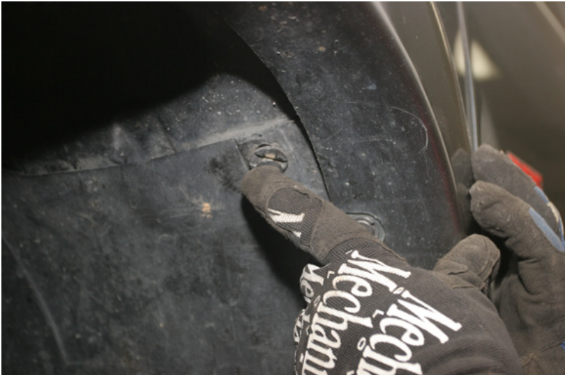
Step 14: The inner wells are installed and the push fasteners are pushed in.
