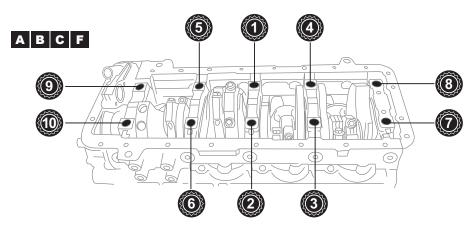
Lubricate Flat Washers (E) and M12 Cross Bolt (D) threads with Lubricant (F). Install Flat Washers (E) on to M12 Cross Bolts (D). Thread assembly into the block. Tighten M12 Cross Bolts to torque spec = 90 ft lbs.
