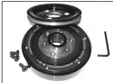
For other FE engines, remove pulley using 6 mm hexagonal wrench.
