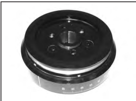
Out of the box damper is set up for use on a 427 or other FE engines with one pulley.
