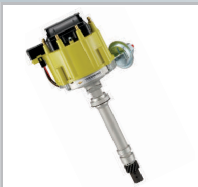
141-681..... Yellow cap HEI Distributor with Coil
