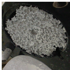
Unprotected and premature transom & outdrive zinc loss
