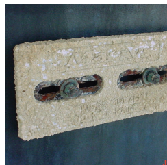
Unprotected and premature transom & outdrive zinc loss
