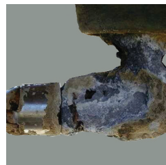
Unprotected sail drive
