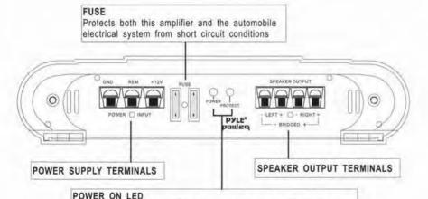
Lights up when the amplifier is energized indicating the unit is on
