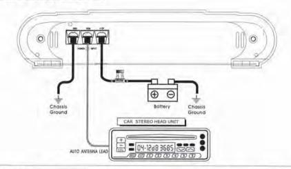
IMPORTANT! Before making any connections, disconnect the car's battery until the installation is completed to avoid possible damage to the electrical system
