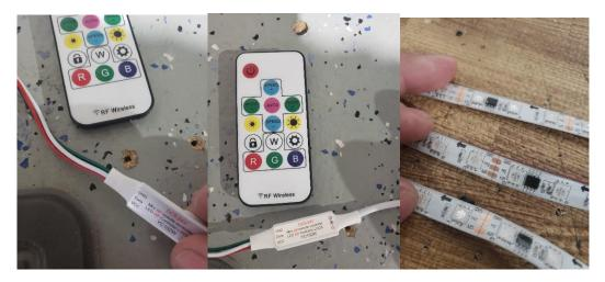
When cutting and soldering wires make sure pattern, arrows are facing the same way if one strip pattern arrow is backwards the chasing feature and the strips would not function properly and would be stuck on one color only. Wires from module are as follows Red is 12volts, White is Ground, Green is data for the patterns.
