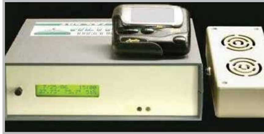
A. ALTACOM II DISPLAY CONSOLE, PAGER, AND REMOVE SENSOR STATION.
