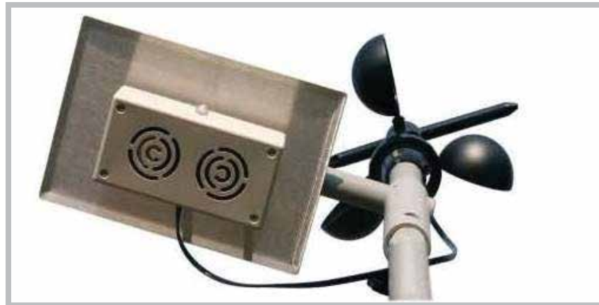
A. THE REMOTE SENSOR HOUSING IS MOUNTED ON THE PVC MAST UNDER THE ALUMINUM SOLAR ROOF. ALSO SHOWN IS THE OPTIONAL ANEMOMETER WHICH PROVIDES WIND SPEED AND WIND DIRECTION.
