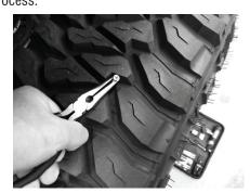
Place a small amount of rubber cement on the T-Handle Reamer tool. The cement will act as a lubricant during repair and help seal the puncture when it dries.
