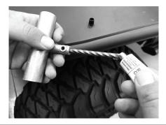
Insert Reamer in puncture. Cycle the reamer through the puncture wound while twisting the reamer. This will open the rubber slightly while repositioning the steel belts to make room for the plug.
