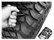
Thread a plug through the T-Handle Insertion Needle. Adjust needle to middle of the plug. Flattening the end of the plug will help get it started through the needle.
