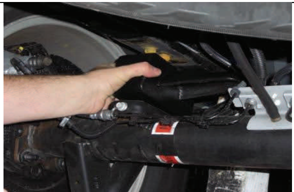
Install lift block with centering pin toward axle.
