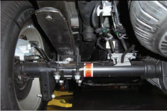
View of 2WD rear axle and leaf springs.
