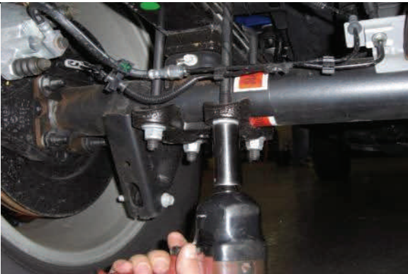
Loosen and remove factory u-bolt hardware.
