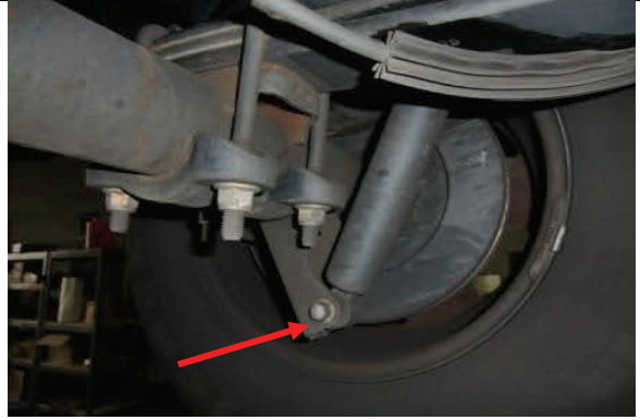
Work on one side at a time and remove lower shock bolt
