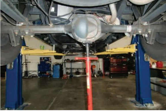
Raise vehicle at frame and support axle with jack
