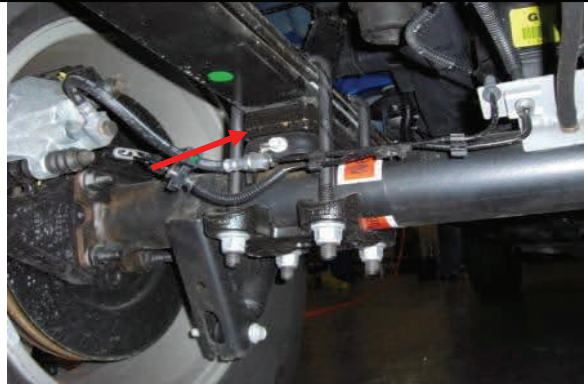
View of 4WD rear axle and leaf spring, note factory block
