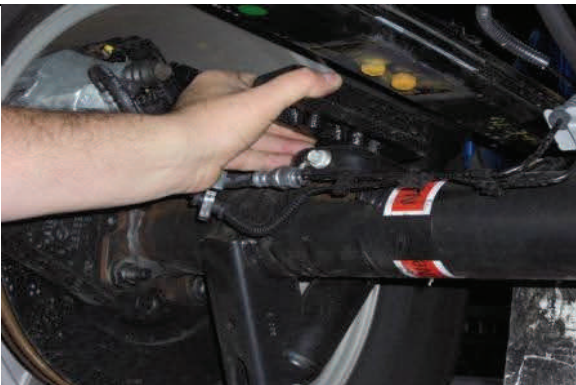
4WD only: Lower axle enough to remove factory block.
