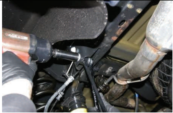
Disconnect upper sway bar end links.
