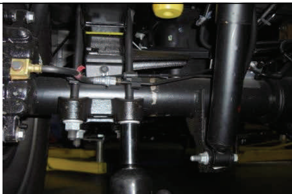
Remove U-bolt nuts and axle mounting plate.
