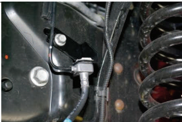
Reinstall block into bracket with retaining clip.
