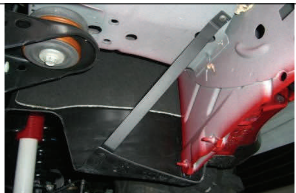
(05-10) Install fender liner strap to clear larger wheel/tires
