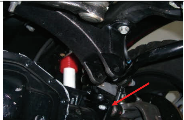
.(05-10) Re-attach and tighten sway bar end links.
