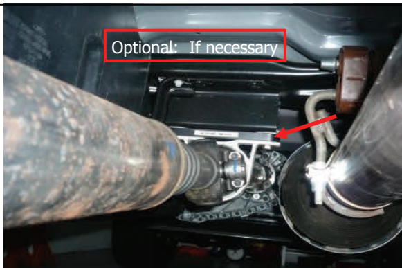
With vehicle on the ground install carrier bearing drop plate.
