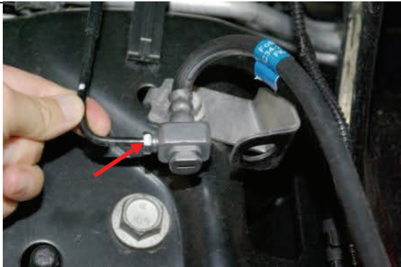
Loosen hard line ferrule rotate block 180 degrees and tighten
