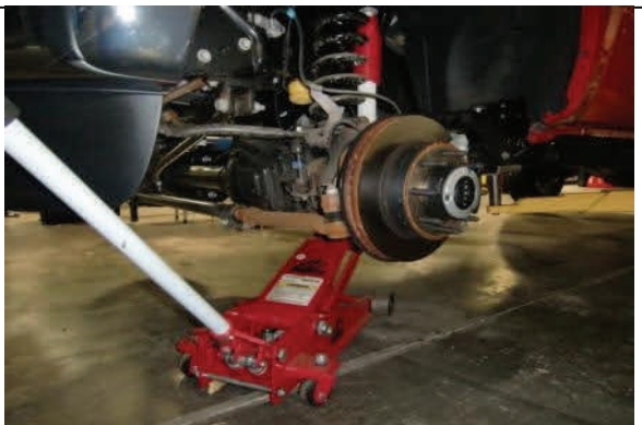
Support front axle with floor jack(s).
