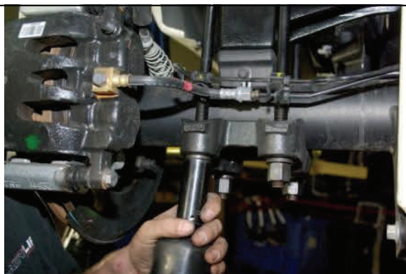
.Install longer U-bolts and nuts onto axle plate. Torque later.
