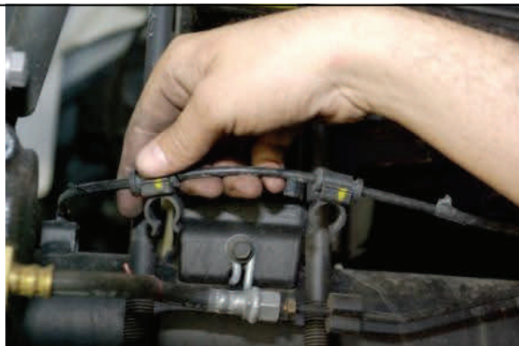
Vehicles with ABS/TC remove clips from U-bolts.
