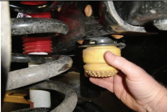
Remove bump stop and unbolt bracket from frame.
