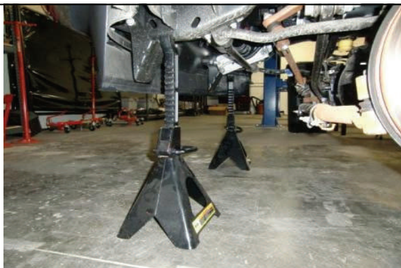
Lift front of vehicle and support with min. 3 ton jack stands.
