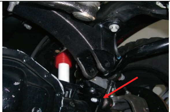
.(05-10) Re-attach and tighten sway bar end links.
