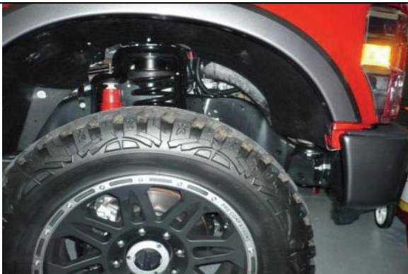
Reinstall wheels/tires, lower vehicle and torque to spec.
