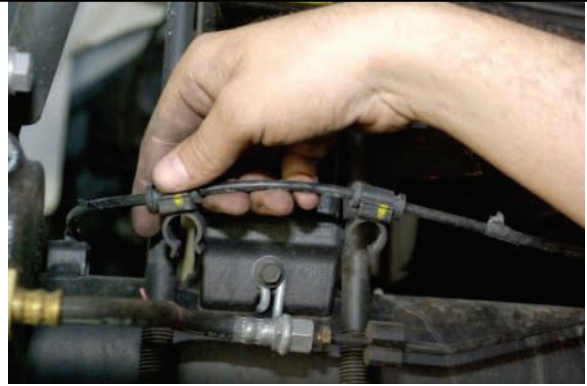
Vehicles with ABS/TC remove clips from U-bolts.
