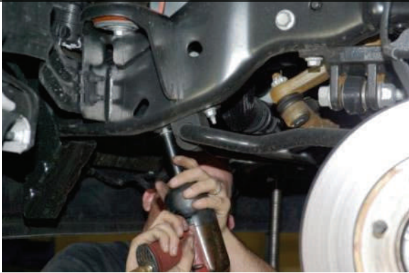
(11-up next 3 steps) Disconnect sway bar at frame and lower
