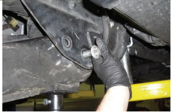
Support radius arm and remove attachment bolts
