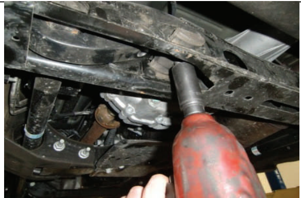
Adjust torsion bars to approx ride height
