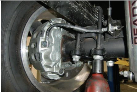
Loosen and remove u-bolt hardware
