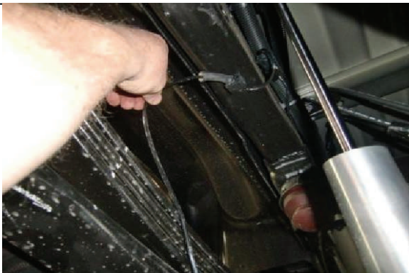
Slide ABS wire clip at frame to gain slack to avoid damage
