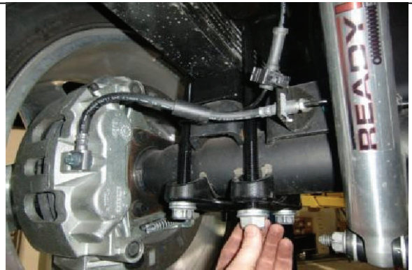
Install new longer u-bolts and install new hardware,
