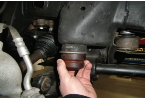
Remove factory lower control arm bump stops (4)
