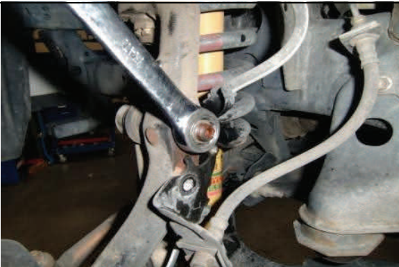
Disconnect sway bar end link at spindle
