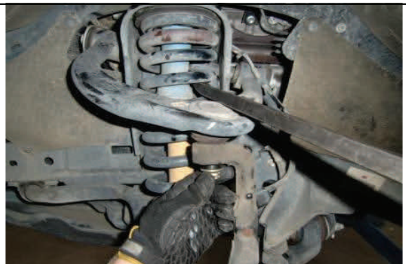
Support suspension and remove upper ball joint nut
