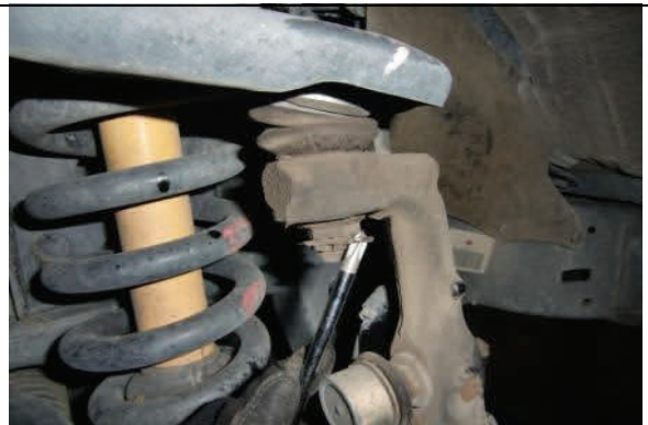
Remove Upper ball joint retaining clip
