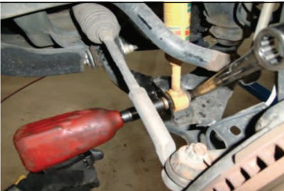
Remove lower strut mounting hardware
