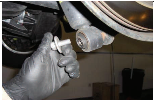
Reconnect and tighten lower shock and sway bar endlinks
