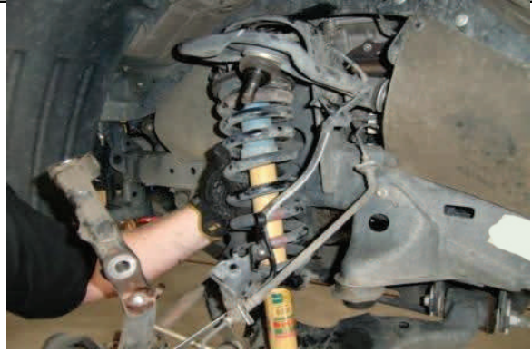
Remove strut assembly from vehicle
