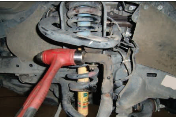
Loosen upper ball joint nut and strike to disconnect
