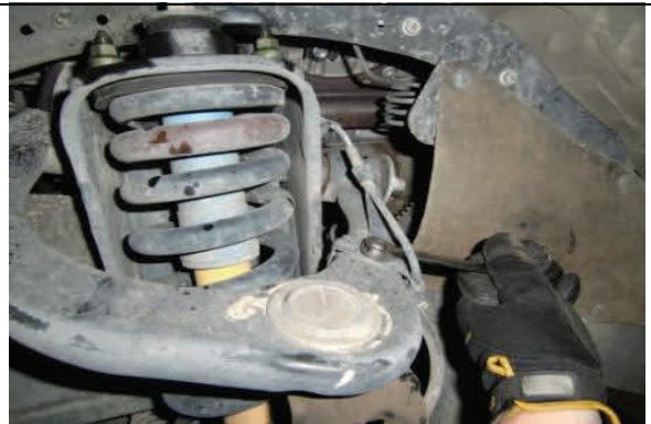
.Disconnect ABS/brake line upper bracket
