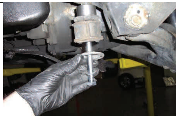
4WD Install longer bolts and reattach differential to frame
