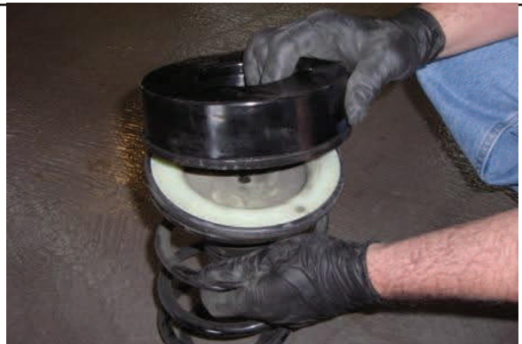
Place coil spacer on top of bump stop on coil spring
