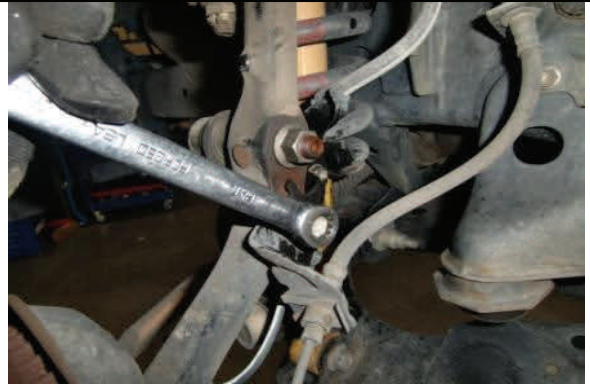
Disconnect ABS/brake line bracket at spindle
