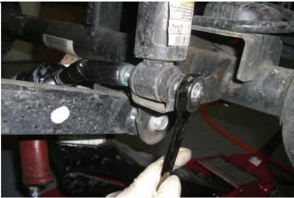
Disconnect and remove front lower shock hardware.
