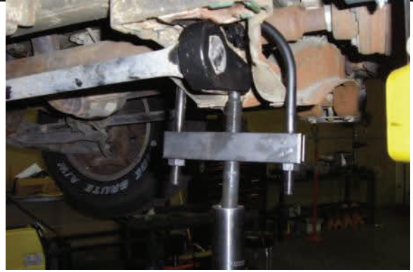
Adjust torsion key tool enough to replace keeper block
