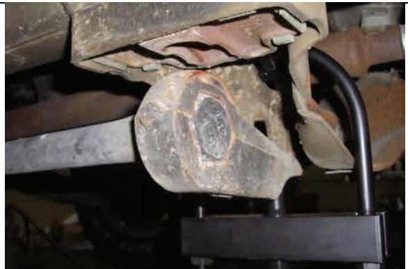
Unload tool and torsion bar will lower, remove torsion key
