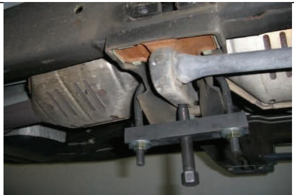
Attach u-bolt over cross member and install tool
