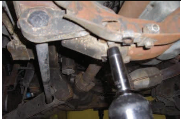
Remove torsion key adjuster bolt
