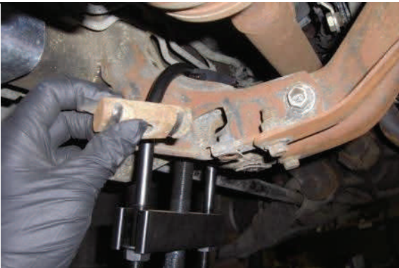
Adjust tool enough to remove keeper block
