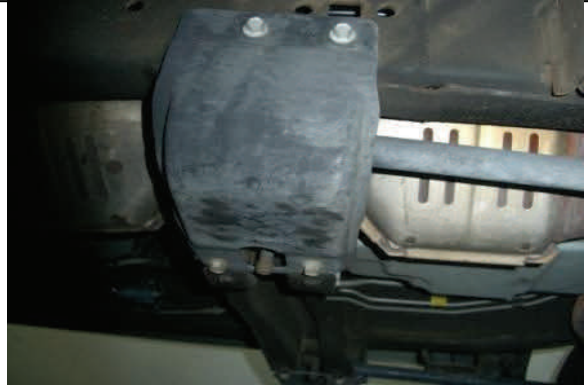
Locate cross member cover and remove bolts
