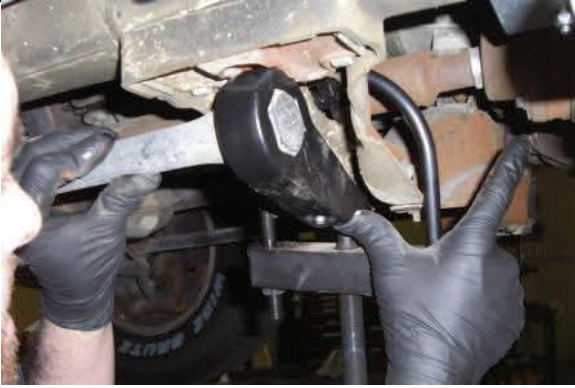
Install new torsion key and reload tool
