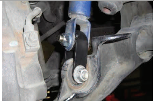
66-3000 Install front lower shock extensions and hardware
