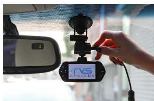
STEP 4: Connect power cable from cigarette lighter to dash camera.
